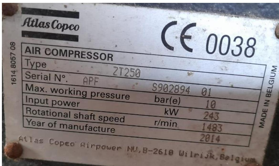
Figure: Utility Air compressor technical datasheet.
