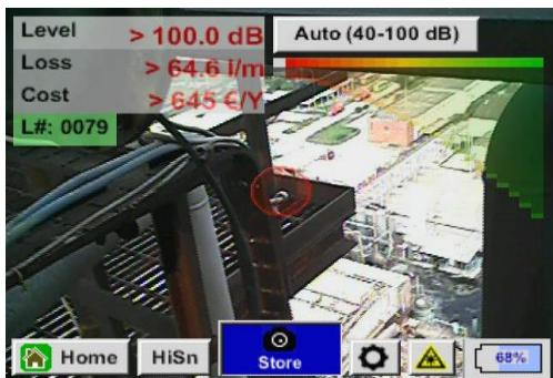
Leakage roof of prilling tower
