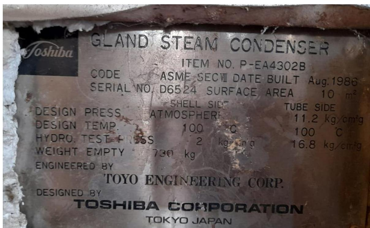
Figure: Steam turbine gland steam condenser technical datasheet.
