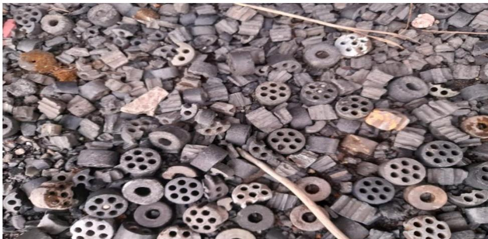
Figure 50: Deactivated and broken catalyst.
