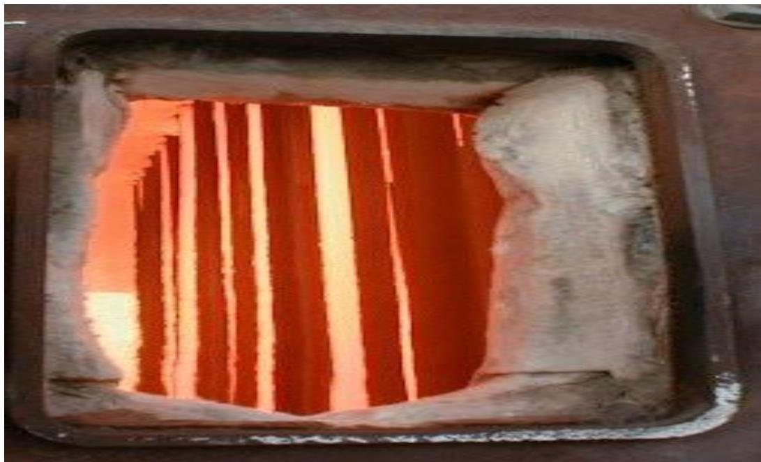
*Figure 35: Sample of localized high temperature of tube surface*
