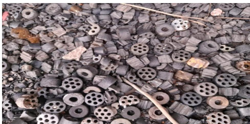
*Figure 34: Deactivated and broken catalyst.*
