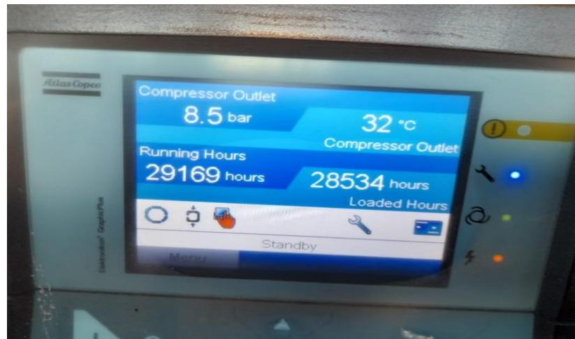
*Figure 32: Air compressor operating hours*
